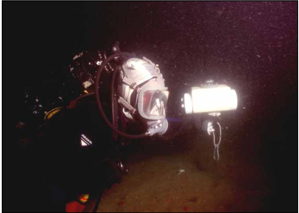
Figure 6-3. Explosive Ordnance Disposal Diving. An EOD diver using handheld sonar to locate objects underwater.
